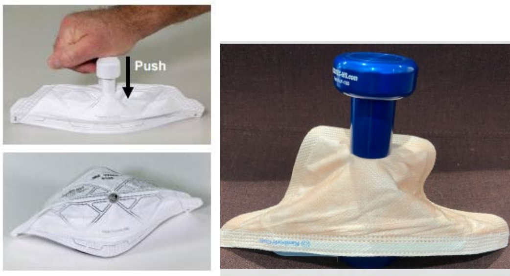
FIGURE 17: USE PORTACOUNT™ PUNCH OR ACCUFIT™ PIERCING TOOL TO INSERT THE PROBE AND NUT
